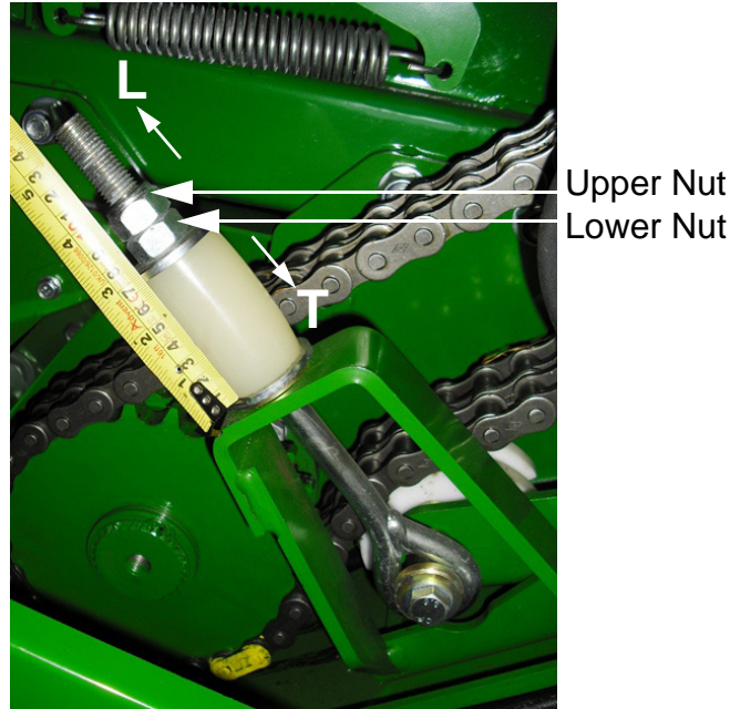
Figure 10.q - Chopper unit duplex chain adjustment
