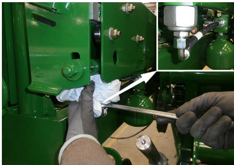
Figure 8.k - Release hydraulic pressure from accumulators
