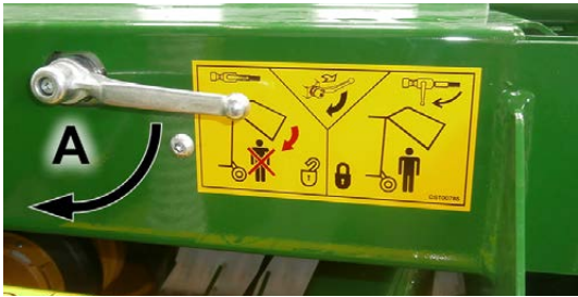
Figure 10.g - Tailgate safety lock
