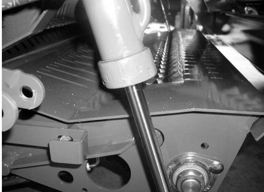
Figure 10.e - Unblock mode, knives retracted and channel floor lowered
