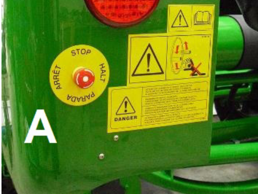
Figure 3.a - Stop switch A located on back left hand corner of back left panel
